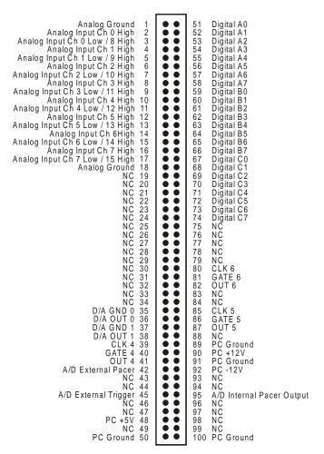
PCI-DAS1000 Connector Diagram
